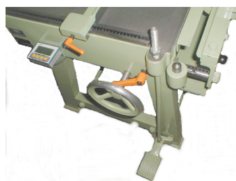
Digital-Display for adjustable for front detent and narrow cutter
